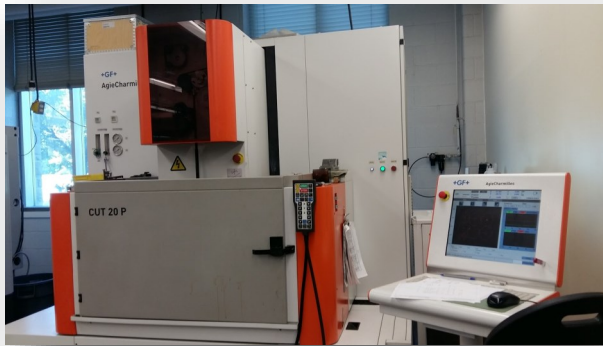
Electronic Discharge Machine (EDM) cuts solid metal into precise shapes.
